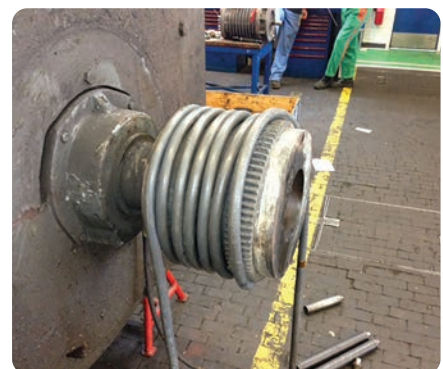
Heating a coupling for dismounting
