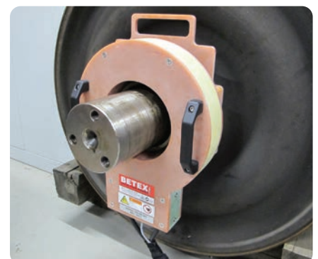
Heating labyrinth rings for dismantling
