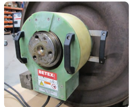
Heating bearing rings for dismantling
