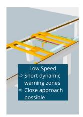
KY-XTRA B.10.01 with digital output signals based on defined distance warning thresholds
