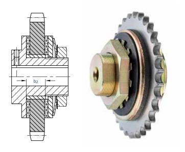
For more precise torque setting and for applications where slippage may be frequent, use a ground center member (63 micro-inch). Rated torque capacity can only be obtained with dry friction facings and with a ground center member, which has been run-in for 4 minutes at approximatley 65 rpm at a torque setting of 70 to 80% of the 1 spring
